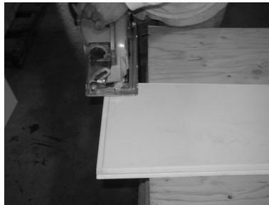
2) Trim shaft pieces to 2¼" shorter than opening—2" for cap/base, ¼" for expansion (¼" if not using cap and base—each part is 1" thick.) Always trim from bottom ONLY—top is marked.
