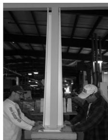
8) Slide assembled 3-sided column around support (on top of base platform).
