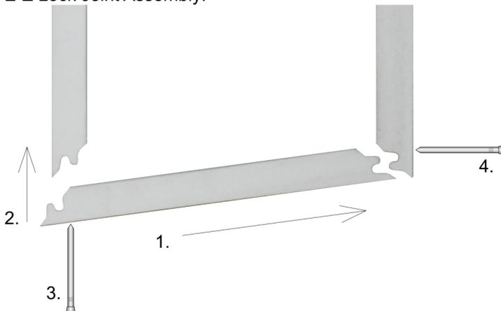
Please note the correct assembly of the E-Z Lock joint shown at the left. Nails **MUST** be installed only in the edges shown (3 and 4). Installing on the other edges may result in open seams.
